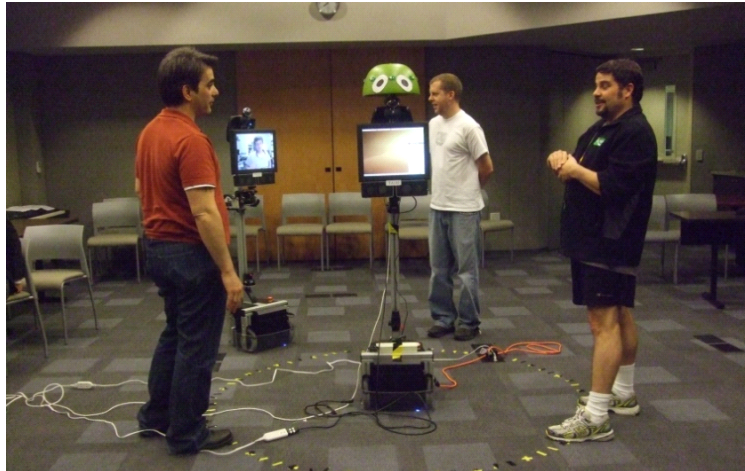
Figure 1.10: A remote operator interacts with two speakers and one Texai through Texai (center). This demonstration was performed in California (CA), Texai on the left was operated from Indiana (IN) by remote control.
