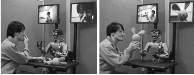
Figure 1: Infanoid engaging in eye-contact (left) and joint attention (right) with a human interactant.
