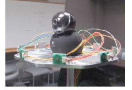
Fig. 5. First version of head: An aluminium disk with 8-channel microphone array on its edge
