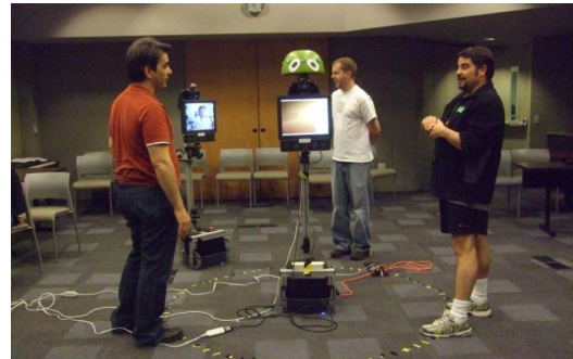
Fig. 1. Three people and one Texai talking around an audition-enhanced Texai in California. In this snapshot, two people are talking together, while the third person is talking to the Texai of which operator is in Illinois.
