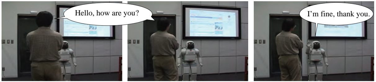
a) A user says a greeting to a robot. b) His greeting was made while in motion. c) The robot correctly responded.
