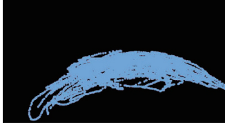
Fig. 4. Drawing of body babbling: NAO’s arm is randomly controlled using the joint angle space. Therefore, most of the drawing consist of arcs.
