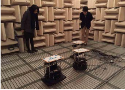
Fig.3 Experimental condition in an anechoic chamber. There are two sound sources (people) and three robots with 8-ch microphone arrays.
