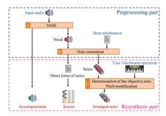
Figure 4. Overview of the proposed system: Inputs are indicated by blue letters and outputs are indicated by red letters.
