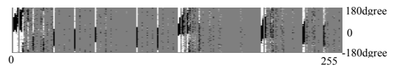
Figure 11: Sensory-behavior space. Vertical dots; a case of vision bumper pattern (256). Horizontal dot; safe direction to move (5 degrees/dot). Black; not safe to move, White; safe to move. Gray; no data.
