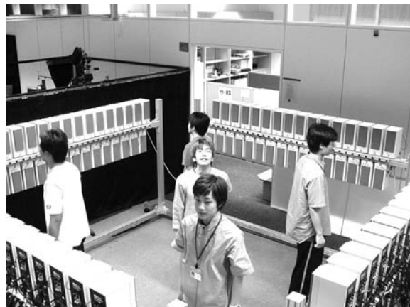
Figure 8: 128-channel square speaker array
