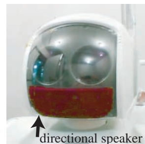
Figure 2: Directional Speaker installed in ASIMO
