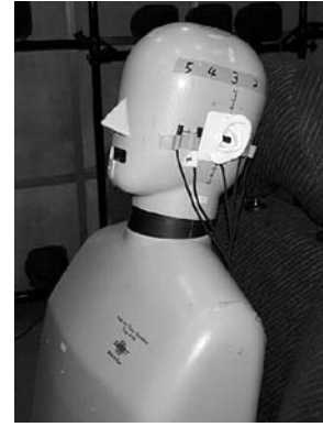
Figure 5: 実験で用いた Head And Torso Simulator
