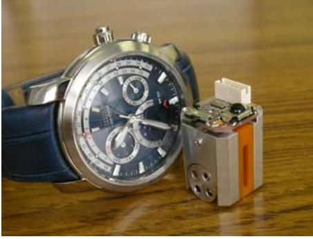
Figure 1: An Eco-Be! prototype. In this robot the differential wheels are driven by two motors which are battery-powered. Besides the PIC controller all other hardware comes from devices originally designed for CITIZEN watches.
